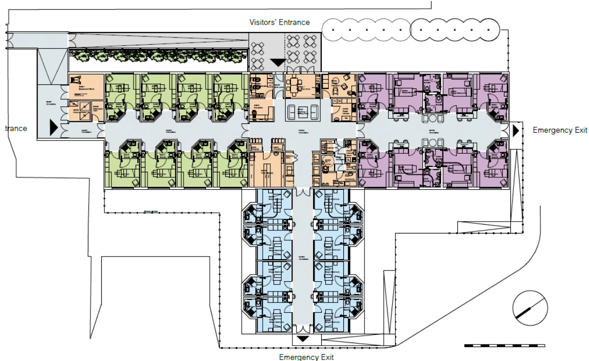
Figur 40 The Hillingdon Hospital, Single Room Pilot Ward
