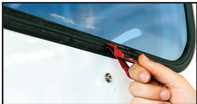
Open emergency exit windows (Pull strap, push window inside)
